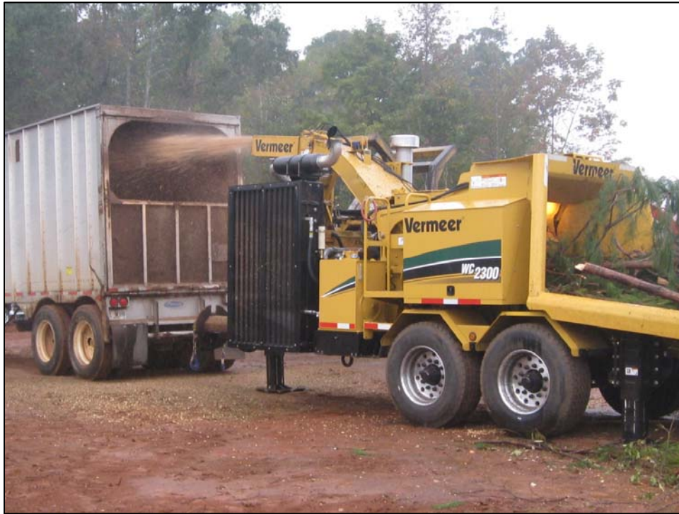
Figure 6. Trailer for whole-tree chips, with opening for chipper to blow chips into.
