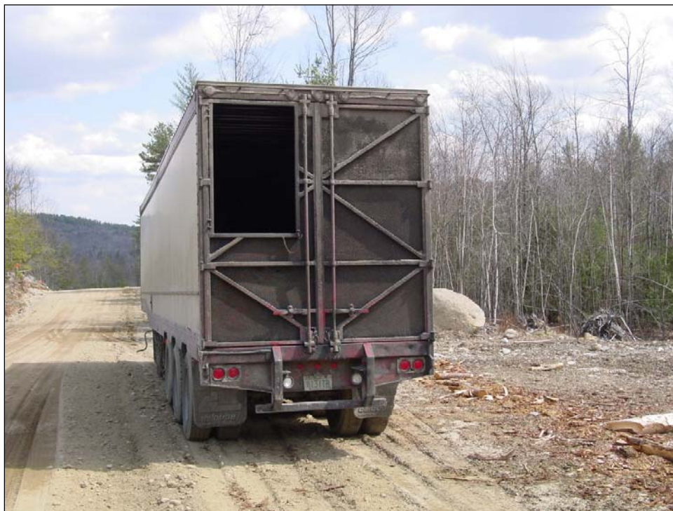
Figure 6. Trailer for whole-tree chips, with opening for chipper to blow chips into.
