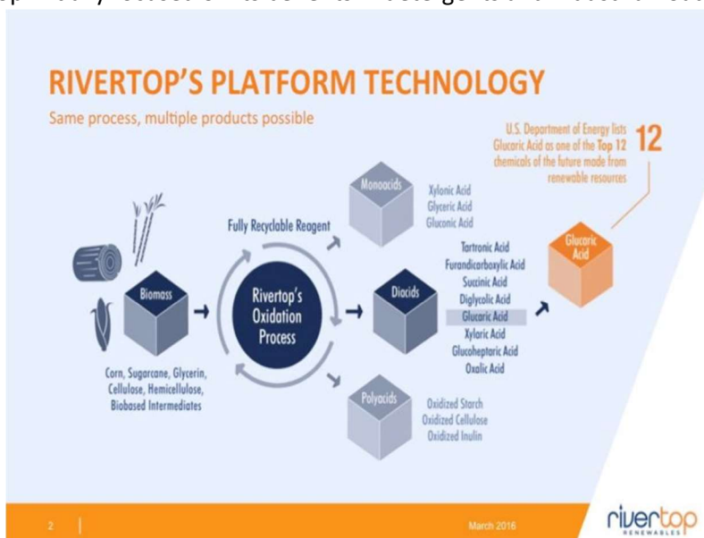
Figure 18: Rivertop's Oxidation Process 61
